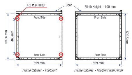
Note: A minimum of 20 cm clearance is required at rear of the cabinet.
