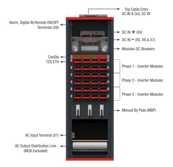
Note: Bravo ECI 72 kVA system is designed as top cable entry
