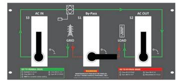
Manual By-Pass puts the module in OFF state but doesn't disconnect the DC. Make sure DC is disconnected before any intervention inside the system.
