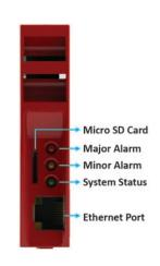
Note: Operation of T2S ETH is described in separate manual available on request.
